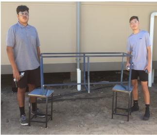
workshop. This has involved Lincoln measuring the new sink, marking out and cutting materials. Tyron and Chris Daniel then laid out the steel box section, tacked it up and welded the leg and rail construction. The three boys then ground the frame up using an electric grinder. After a quick file for ergonomics, coat of primer and ocean blue top coat, the boys have completed their first independent project for the
